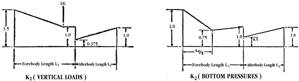
FIGURE 4b-15b—Hull station weighing factor.
