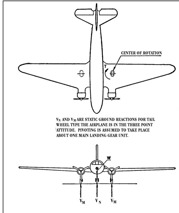
FIGURE 4b-14—Pivoting, nose or tail wheel type.
