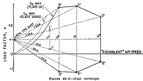
(2) *Design maneuvering speed,  $V_A$ .* The design maneuvering speed  $V_A$  shall be equal to  $V_{S1} \sqrt{n}$ , where  $n$  is the limit maneuvering load factor used (see § 4b.211(a)) and  $V_{S1}$  is the stalling speed with flaps retracted at the design take-off weight. (See fig. 4b-2.)
